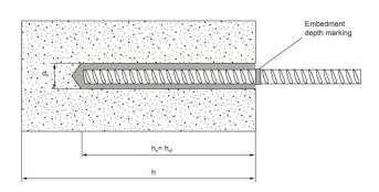
Table A2: Installation details for rebar
